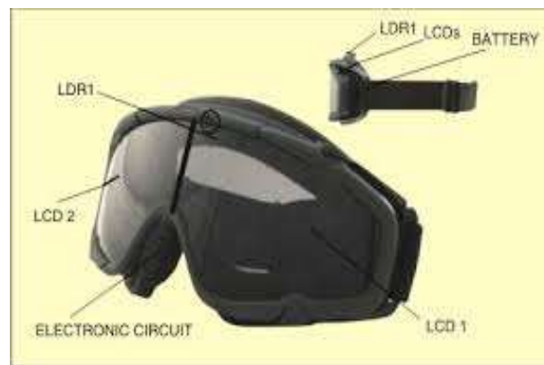
Figure 5 : Circuit fitted on transparent LCD's
